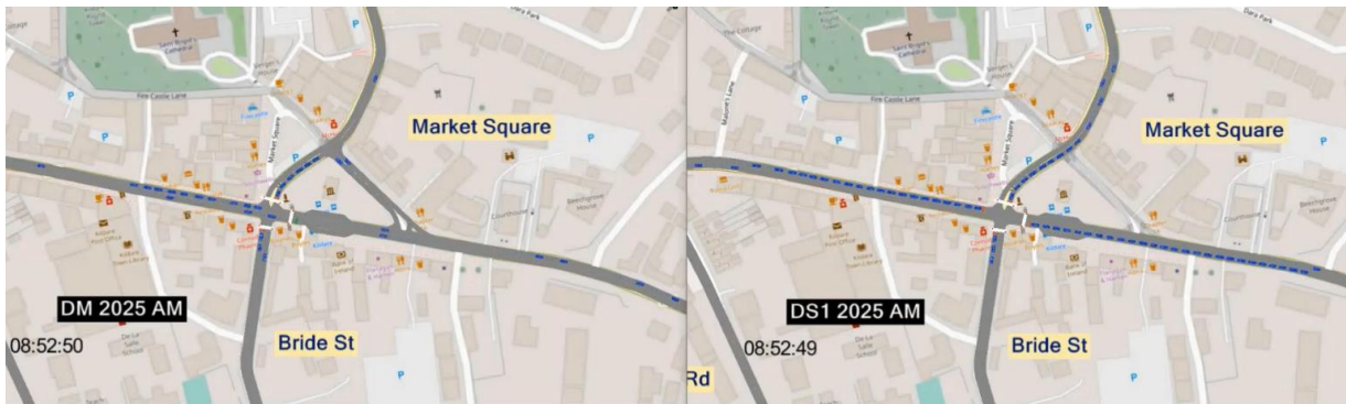
Figure 3.8 VISSIM 2025 AM – Comparison of DM and Eastern Section of Market Sq. Closed to Traffic
